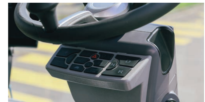
Control panel on the steering column The control panel contains all driving relevant buttons, easily and quickly accessible.
